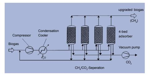
Schematic flow sheet for upgrading of biogas to vehicle fuel standards with carbon molecular sieves.
